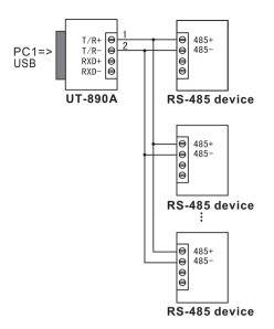
3. Half duplex connection between UT-890A interface converters
